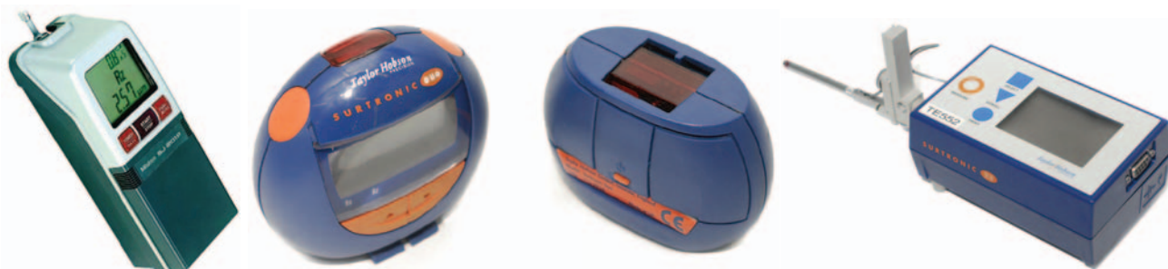
Figure 3 Surface microroughness meters (left to right: Mitutoyo SurfTest SJ201P, Surtronic Duo, Surtronic 25)
